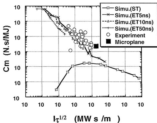
Fig.2 Dependence of  $C_m$  on  $I\tau^{1/2}$ . ST indicates the standard target which is the single layered target, while ET indicates the exotic target which consists of a metal layer over-coated with transparent material. The open circles show the experimental result achieved by LHMEI laser, and the closed square represents the result of the micro-airplane. In the simulation, the pulse width of the laser was varied from 5 ns to 50 ns.
