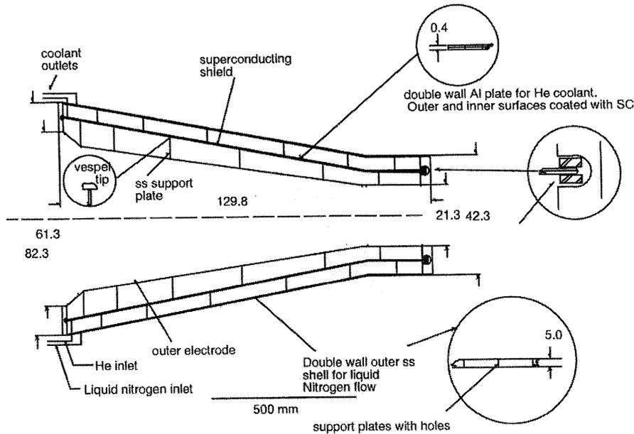
Fig. 3 Reference design for the superconducting shield for the JT-60U CT injector.
