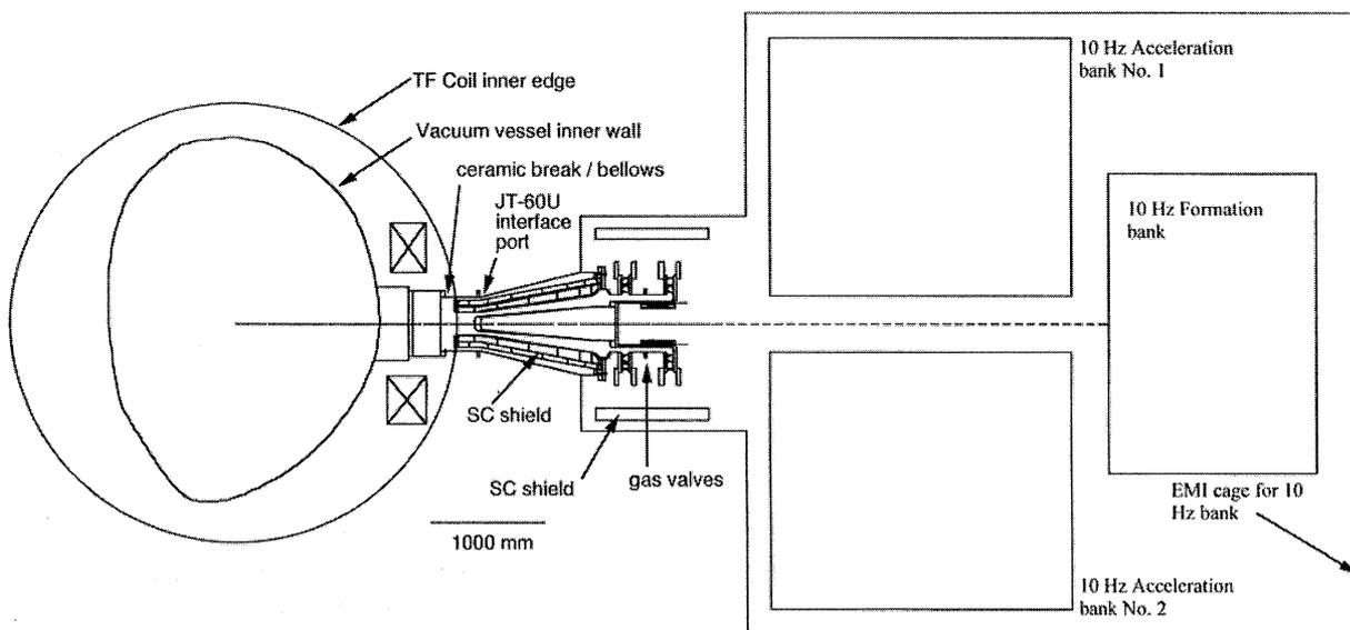
Fig. 2 Schematic of CT injector layout for JT-60U.
