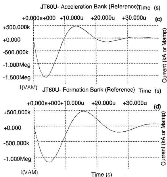
Fig. 4 Circuit currents from simulation using the Spice circuit simulation code for the Acceleration and Formation stages.
