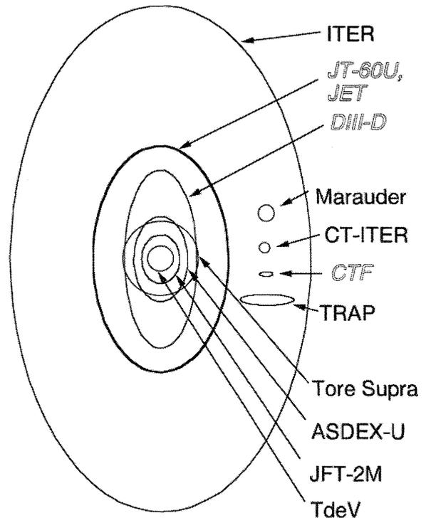
Fig. 1 Relative minor cross-sections of various tokamak plasmas and of compact toroid plasmoids. Note that injection of CTF sized CTs into DIII-D or JT-60U sized plasmas will result in localized fueling at reduced level of perturbation to the target tokamak.
