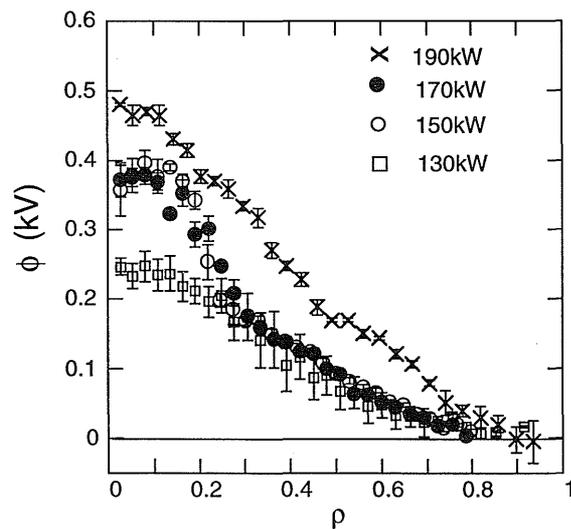
Fig. 1 Dependence of potential profile on ECH power. A threshold is shown to form a potential profile with a protuberance. The square, open circles, closed circles and x-marks represent the potential profiles with ECH power of 130 kW, 150 kW, 170 kW and 190 kW, respectively.
