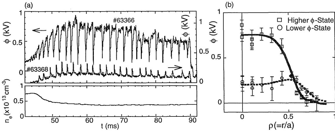
Fig. 3 (a) Pulsating behavior of the potentials at the center and at an outer radius of  $\rho = 0.59$  in CHS plasmas. This phenomenon is referred to as electric pulsation. The example is observed in a combined ECH+NBI heating phase. The time evolution of the line averaged electron density, that was measured with an HCN interferometer, is shown below. (b) The potential profiles of higher and lower potential states. Here  $\rho$  is the normalized minor radius.
